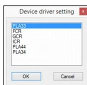
Select the appropriate instrument from the list and confirm by pressing the button OK. Then the device will be added to the list. Now it is necessary to define the ID of device in RS485 bus and communication interface used for connection to PC.
