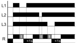
If all three phases are available, red LED is Off and output relay is open. If any of phase is missing (voltage level under set **Umin**), then after set time delay output relay disconnects and red LED starts blinking. Type of blinking defines the phase with failure.
