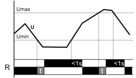
If the voltage in any phase is out of the set level, red LED is Off and output relay is opened. If voltage in any of three phases goes over set **Umax** or below the set **Umin**, red LED starts blinking and output relay disconnects. Type of blinking defines the phase with failure. Time delay settings defines delay of failure detection. If failure is shorter than time delay, the output does not react on it.
