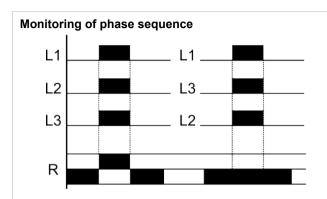
If all three phases are in correct phase sequence, red LED is Off and output relay is closed. If phase sequence will change, red LED turns On and output relay disconnects.
