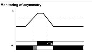
If asymmetry of controlled phases is under the set level, red LED is Off and output relay is opened. If the set maximum level of asymmetry is exceeded, red LED turns On and output relay disconnects.
